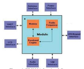
Figure 4. SIM900A functional diagram
