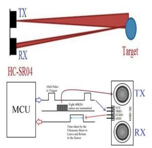
Figure 3. Working of ultrasonic sensor.
